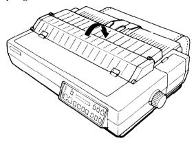
**5.** Press the **ON LINE** button to set the printer on line.
